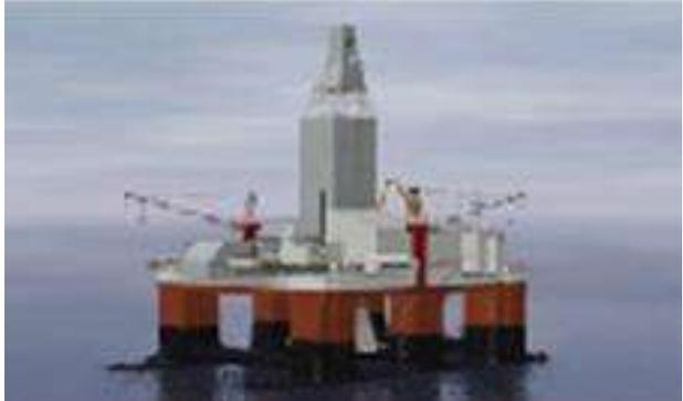
Platforms are equipped with four azipods with FPP.
